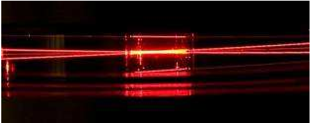
Figure 2: The focused laser beams intersecting in the scattering volume of a sample. http://www.lsinstruments.ch/services/technology/3d_cross-correlation_light_scattering/ Retrieved 06-21-2011
